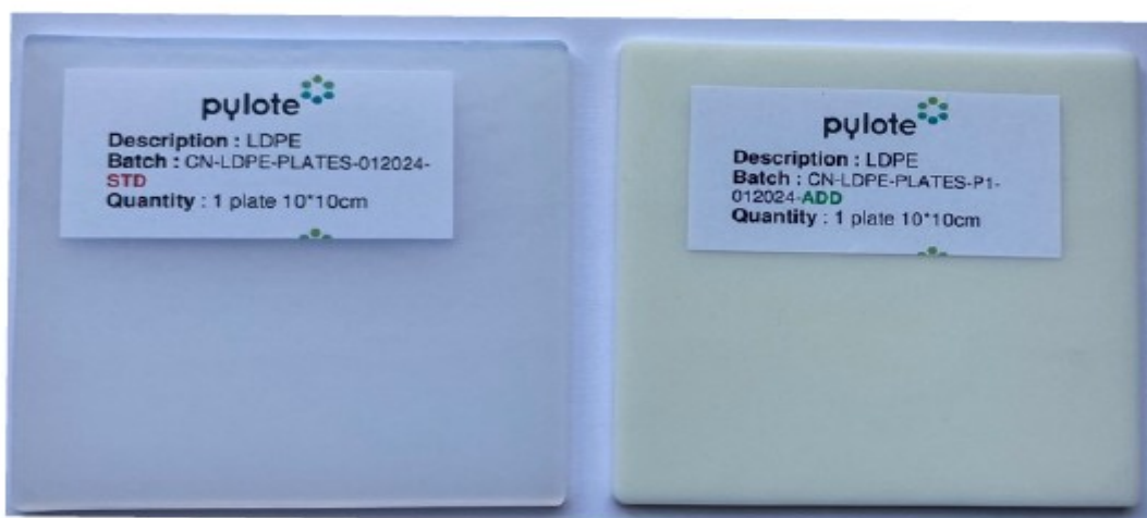
Figure 2. LDPE samples: untreated (left) versus treated (Right) coupons
